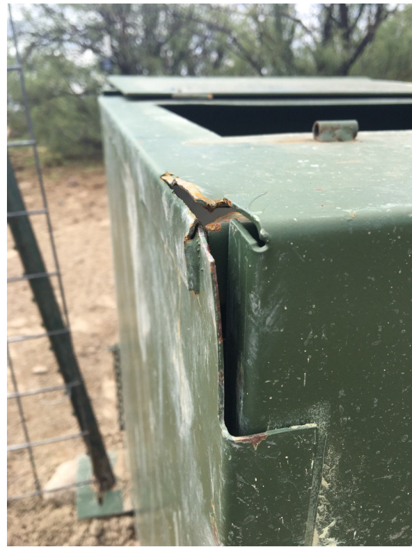
Figure 17: Photos of representative feral hog damage to feeder door pin holes, door track, and lid.
