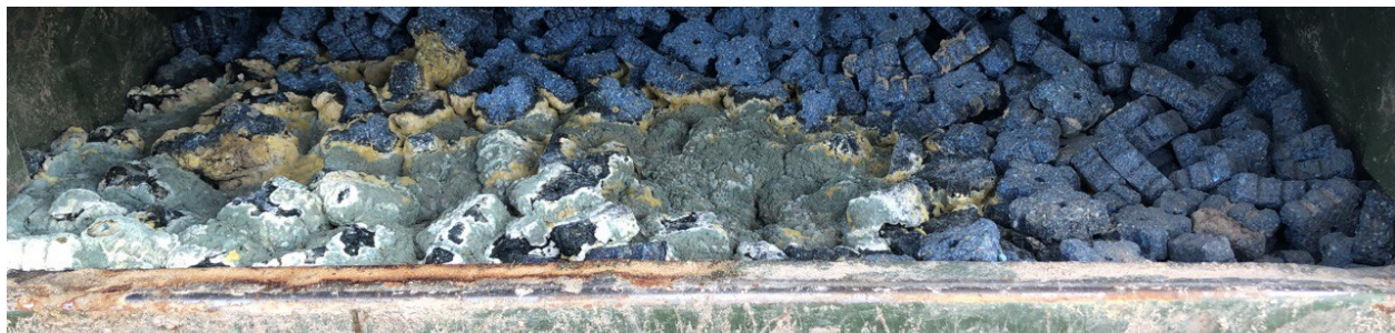
Figure 10: Example of disintegrated and molded Kaput® product when exposed to water long-term.
